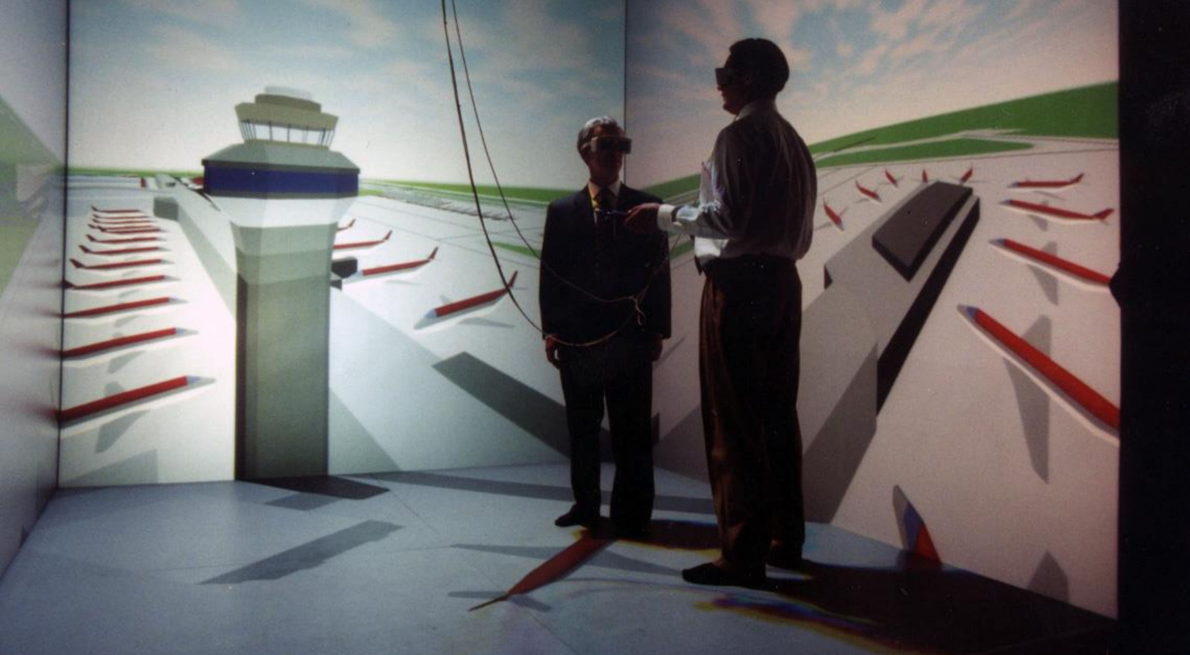
1997: screen resolution 768 × 768 (?); tethered tracking; single primary viewer
